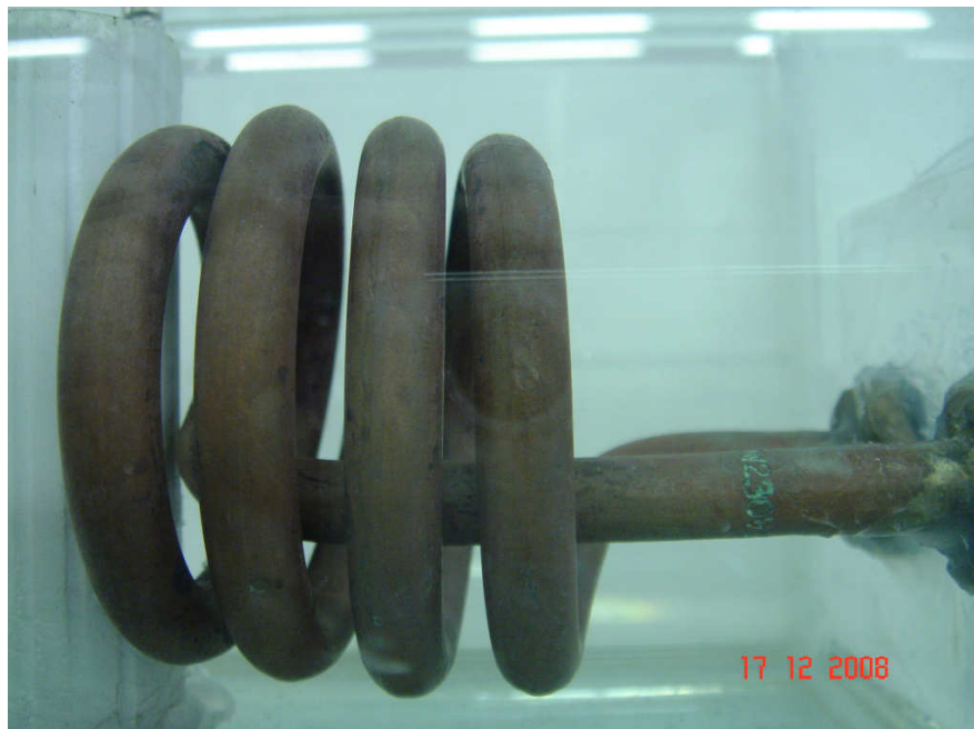
Figure 10.2 – With Aquabion As compared with the coil not protected by AquaBion, this coil corroded for about 10% at the 80 th hours of testing.
