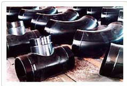
Figure 6.1 – DHF Anti-corrosion treatment and coating
